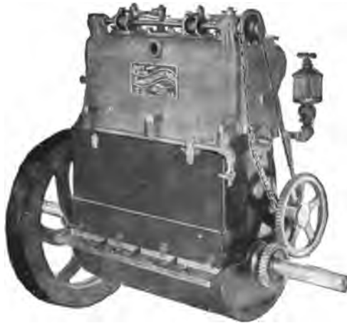
FIG. 306.—Four-Cylinder, 10 H. P. "Buffalo" Gasoline Engine for Motor Vehicle Use. The gearing of this motor renders it non-vibrating, as guaranteed, while, by the "shifting-spark" system of governing, the speed may be varied from 100 to 1,500 R. P. M. without changing the motion of the valves. This is an exceedingly flexible system of governing. The cylinder head is water-jacketed; the firing stroke in the four cylinders follows consecutively, thus securing perfect balance; the inlet valves are positively operated, thus enabling a wide range in adjusting fuel charge ratios. On account of the four-cylinder positive igniters, the engine is very easy to start.
